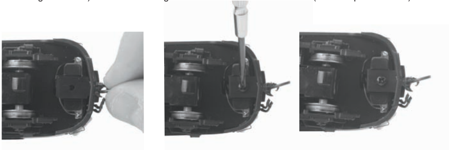
Line Up CENTER Mounting Hole In Coupler Pocket With Mounting Hole On Chassis
