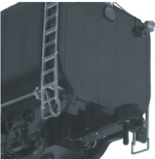
Figure 3: Shorten locking pin when coupler is in lower position..
