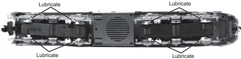
Lubrication Points on the Locomotive
