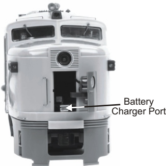
Battery Recharging Port
