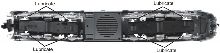
Lubrication Points on the Locomotive
