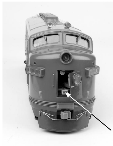
Figure 28: Battery Recharging Port
