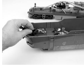
Figure 25: Pulling the lights out of the guides.
