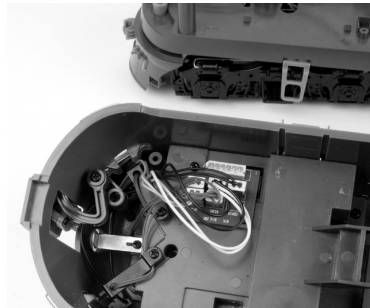
Figure 23: Wire harnesses connect lights inside the locomotive body.
