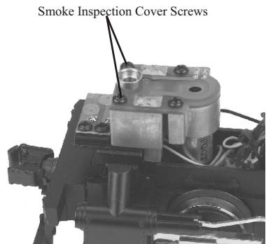
Figure 6: Smoke Unit Inspection Cover
