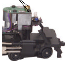
Figure 6. Smoke Unit Inspection Cover
