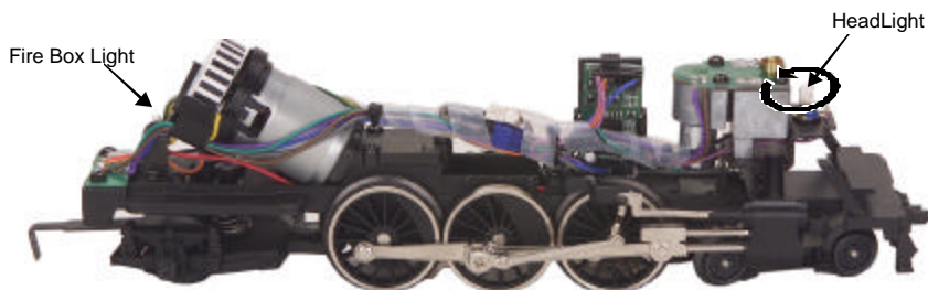
Figure 8. Replacing the Headlight and the Fire Box Light
