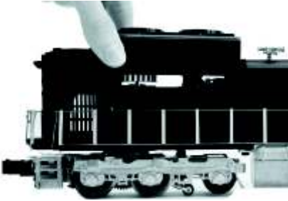
Remove Fan Cover to Access Battery Charger Port
