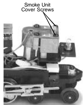
Figure 12. Inspection Cover Screws
