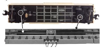
When you are ready to operate the signalman boxcar, make sure the entire car is on the Uncoupling/Unloading Track Section (UTS\*), so that the car's slide shoe pick-ups are in contact with the fourth and fifth rails of the UTS. The recommended voltage for the operation is 12-16 volts.
