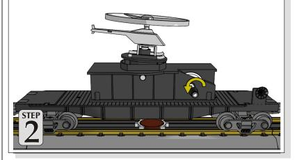
**Taking Off:** Hold the Uncoupling Track Section switch in the "Unload" position. (Refer to your UTS instruction sheet for complete directions in its use.) The helicopter will remain on its base, with blades turning, until you release the switch, at which point it will take off in the direction of the platform's angle. The recommended voltage for the helicopter's flight is 12-15 volts; this will allow the helicopter to fly 5-10 feet.
