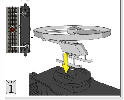
**Determining Helicopter Trajectory:** Insert the small plastic key (included) into the hole on the side of the car. Turn this key counterclockwise to tilt the platform back and forth in the direction you want the helicopter to fly.
