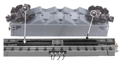
When you are ready to operate the coal hopper, make sure the entire car is on the Uncoupling/Unloading Track Section (UTS\*), so that the car's slide shoe pick-ups are in contact with the fourth and fifth rails of the UTS.
