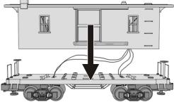
To be able to separate the interior from the shell you need to remove the connector board mounted underneath the interior and unplug the two connectors from the board.
