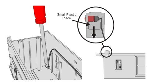
The LED bulb is sandwiched between the lantern and a small plastic piece which will need to be removed also in order to access the bulb. Upon reassembling your caboose, you will need to run the wires for the LEDs in the wire channel that they were originally in (shown in step7). This will prevent the wires being seen inside the caboose.
