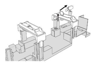
6 In order to change the LEDs located at either end of your caboose, you must remove the lantern assembly from the corresponding end of the LED you wish to change. You will need to take a small screwdriver and push the lantern out from inside the shell (shown in Fig 6).
