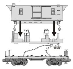
5 You can now replace the bulbs by pushing the socket up from the bulb holder and pull the bulb from its socket. Replace with a new one, and reverse the steps to reassemble the caboose. To replace the two red LED lights at the end of the caboose follow steps 1- 4, above and below, and 6-7 on the back page.
