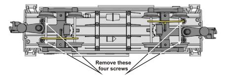
With the four screws removed, lower the chassis from the shell, take care not to
