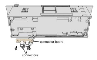
4 Once the board is removed you can then lower the interior from the shell.
