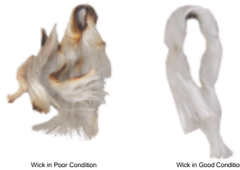
Figure 6. Examples of a wick in poor condition and in good condition.
