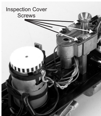
Figure 11. Inspecting the Smoke Unit Wick
