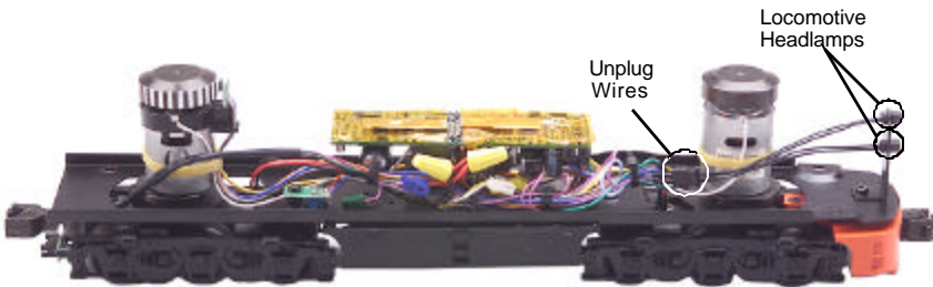
Figure 5. Location of the headlamp in the Engine.
