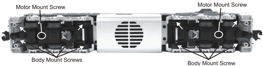
Body Removal Screw Locations
