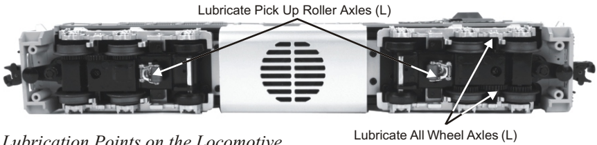
Lubrication Points on the Locomotive
