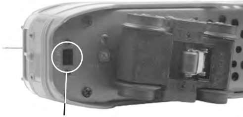
DCS/DCC Switch Location
