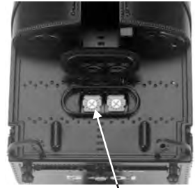
Proto-Sound® 3.0 Manual Volume Control on PT Tender
