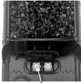
Proto-Sound® 3.0 Manual Volume Control on Tender
