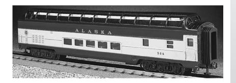
Thank you for purchasing the MTH Premier FLVD Passenger Car. The cars's durable ABS body and die-cast trucks are traditionally sized for operation on most O-42 Gauge curves. The unit should operate for years with any AC transformer and is completely compatible with most 3-rail locomotives, rolling stock and accessories.
