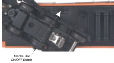
Figure 3: Smoke Unit Switch Location
