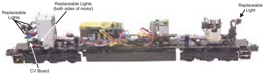
Figure 7b. Replacing the Light Bulbs
