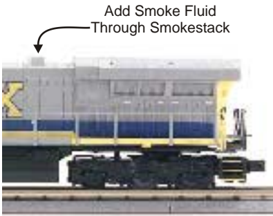
Figure 8. Filling The Smoke Unit
