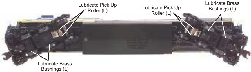
Figure 5. Lubrication Points on the Locomotive
