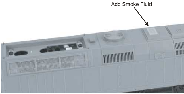
Figure 2. Adding Smoke Fluid
