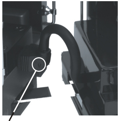
Arrow will point upwards when plugged in correctly
