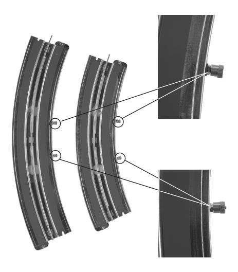
The recommended operating voltage range for the No. 85 Race Car Set is 10-20v AC or DC. Make sure the terminals of the outer track do not contact the inside track.
