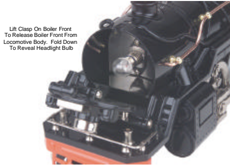
Figure 4: Accessing The Locomotive Headlight
