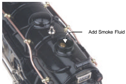
Figure 14: Filling The Smoke Unit
